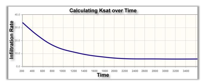
If infiltration rate is plotted over time, the curve will eventually flatten and become constant when the soil has reached 100% saturation. This constant is Ksat.
