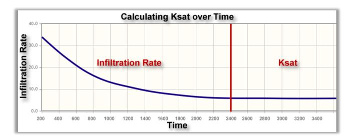
Ksat is the only reliable metric to quantify the condition of an infiltration raingarden and its expected performance during a storm event.
