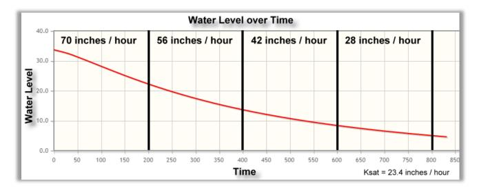
The graph above shows the water drop in a cylinder, over time (seconds). If infiltration rate were calculated every 200 seconds, you can see that infiltration slows down as the ground saturates (see figure below).
